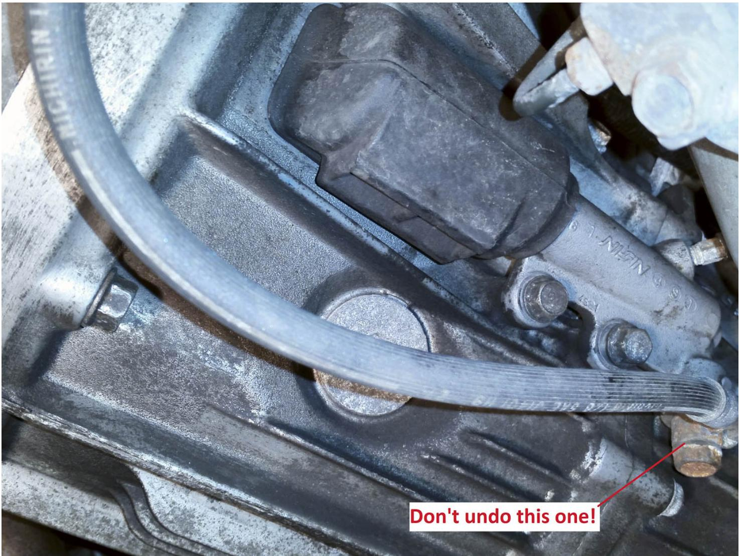
5. On the passenger side of the engine, there is a short ground cable that is screwed to the subframe. I had just enough slack to do the rest of the job without removing one end, but you might not be so lucky. I would remove this from the subframe.
