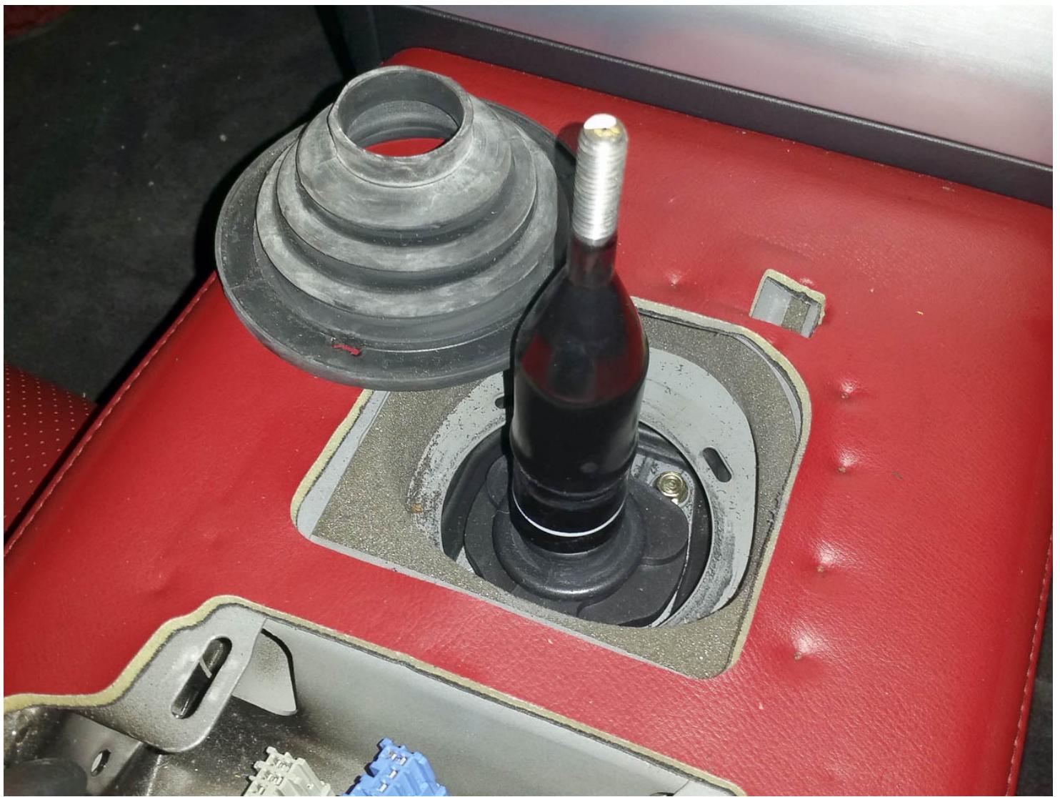
6. Lift the second rubber boot and undo the three 10mm bolts underneath it. Lift the gear lever and remove it.
