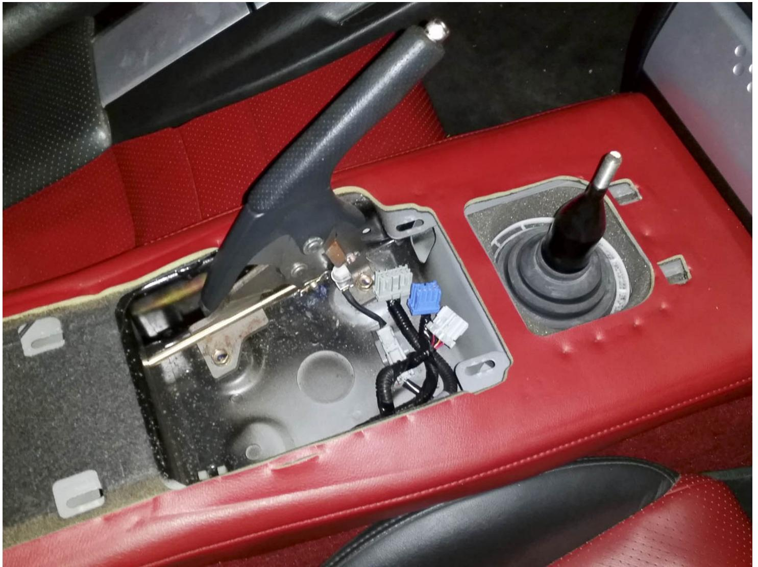
4. Gently put a flat bladed screwdriver into the gaps in the gearstick's rubber surround, between the rubber and the white plastic ring. Push against the white plastic to release each of the 4 tabs. The area of the ring near each tab should gently 'spring up' as it's released. Remove the white ring.
